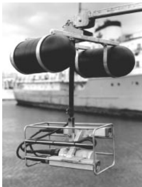
Figure 2: The underwater portion of the Salmon Sizing System showing the two video cameras, with flotation devices at the top.
