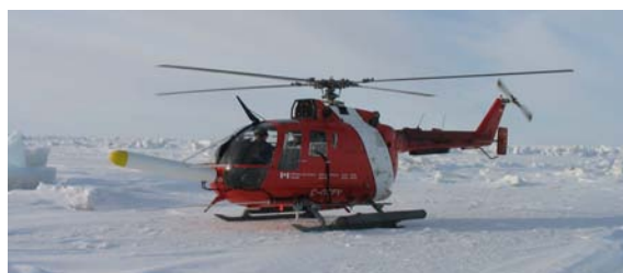
Fig. 1: The IcePic™ sea ice measurement system mounted on a Canadian Coast Guard BO105 helicopter.
