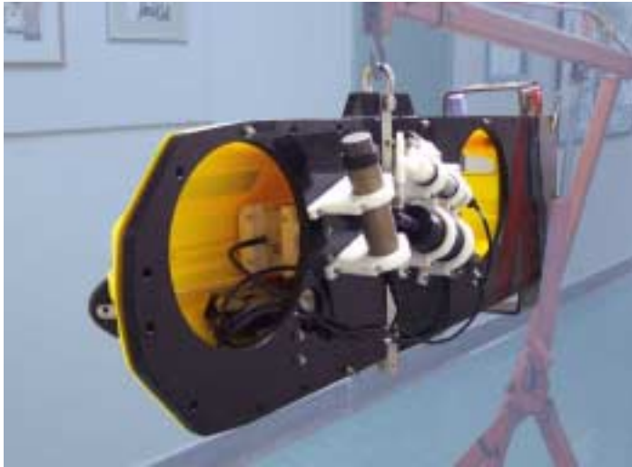
Fig. 2, Sensor float with fairing and buoyancy spheres removed.
