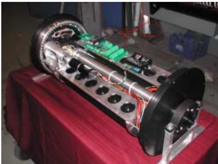
Fig. 7. SeaMotor with winch drum/pressure case removed.
